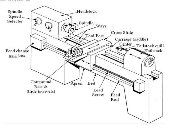
A lathe is a machine tool which rotates the work piece on its axis to perform various operations such as cutting, sanding, knurling, drilling, or deformation with tools that are applied to the work piecetocreate an object which has symmetry about an axis of rotation.
